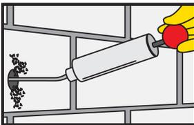
The drill hole must be cleaned with a blow pump or by compressed air, starting from the bottom of the hole. (at least 2x)
