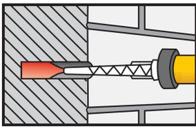
Inject the adhesive into the hole, starting from the bottom, while slowly drawing back the static mixer. In any case avoid entrapping air. For deep holes extension tubing can be used.
