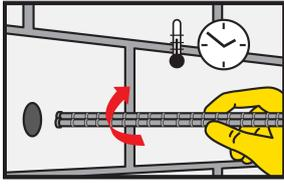
Insert the anchor with a rotary motion into the filled drill hole. Some adhesive must come out of the hole. Important: the anchor must be placed within the open time.
